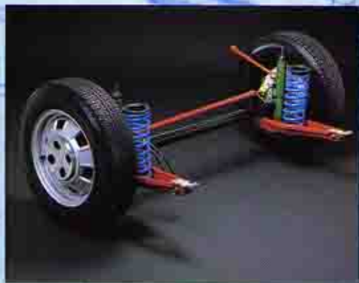
Straight and unsplit rear axle, without heavy power transmission components. Effectively absorbs the irregularities of the road surface. The unvarying track also contributes to a firm grip.
