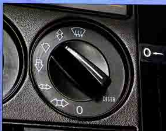
The air distribution control with programmed settings. Seven logically arranged positions. Can be preset quickly, without the need for irritating re-adjustments. Vacuum-controlled dampers and flaps for trouble-free operation.
