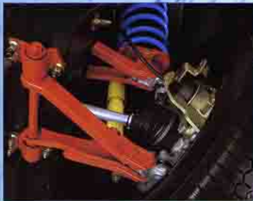
Double wishbones ensure high stability. Excellent road grip, largely due to pivot mounting of the springs which are therefore always straight and fully effective.
