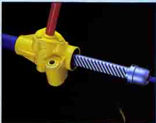
The rack-and-pinion steering gives immediate and distinct response to the slightest movement of the steering wheel. Ideal in combination with front-wheel drive.
