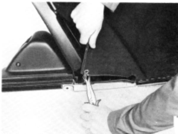
17 Remove the finisher strip from the tail edge of the top.
