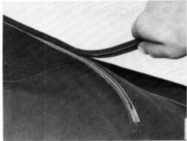
20 Mark the left and right ends of the aluminium retainer strip and remove the strip.
