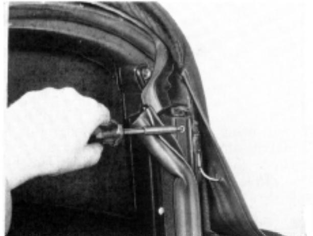
5 Remove the nuts securing the seal retainer to the front section of the side rail.
