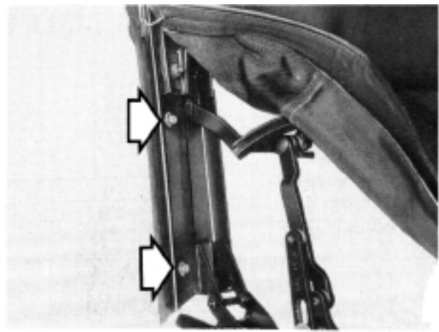
6 Remove the screws in the leading edge of the seal and remove the seal.
